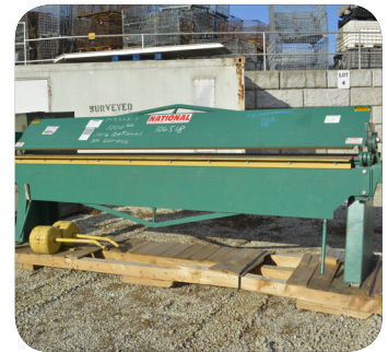
Sheet Metal Brake Can bend 16-gauge sheet metal $1,000
