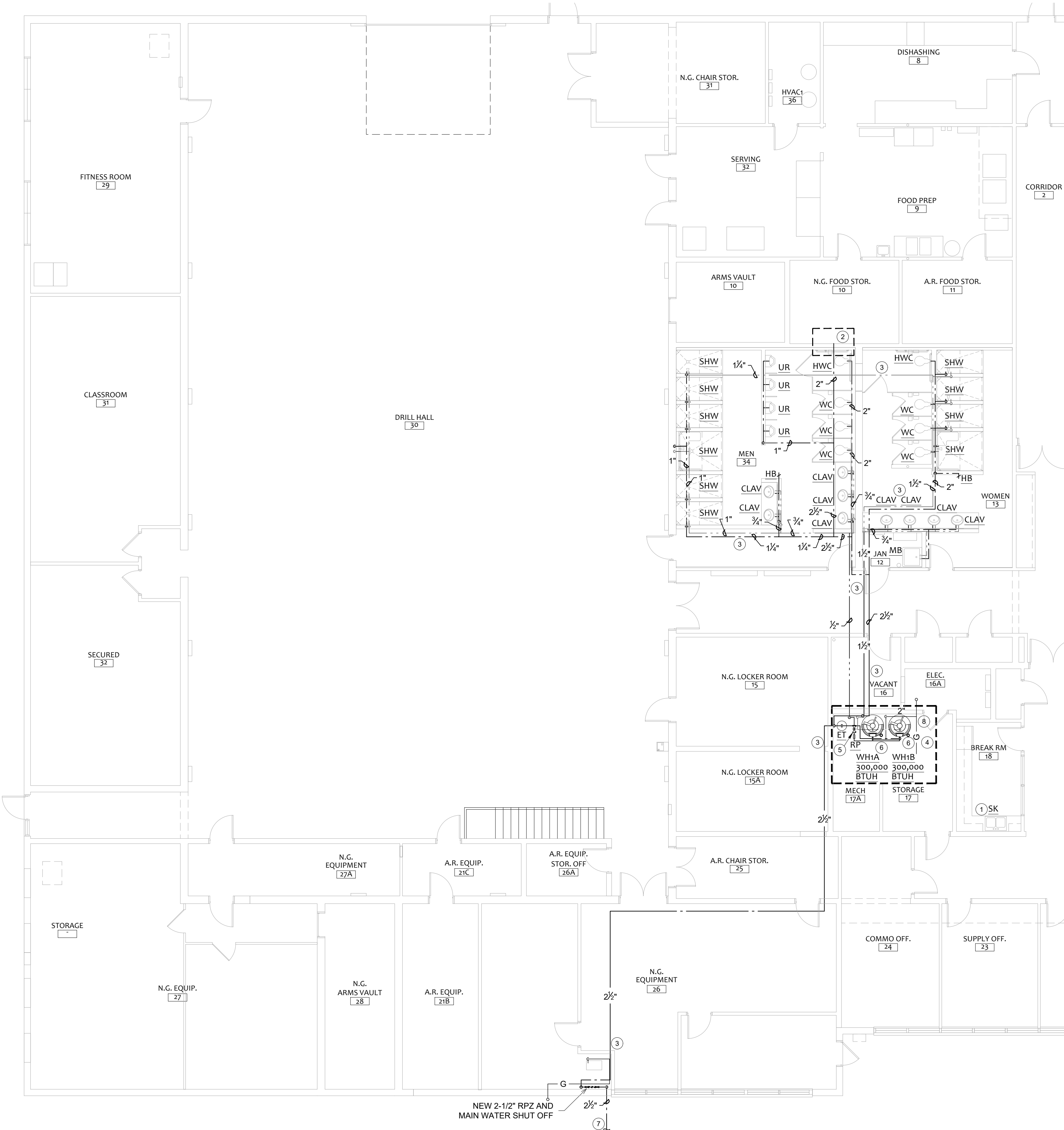
1P-102 SUPPLY PIPING PLAN 1/8" = 1'-0" N
