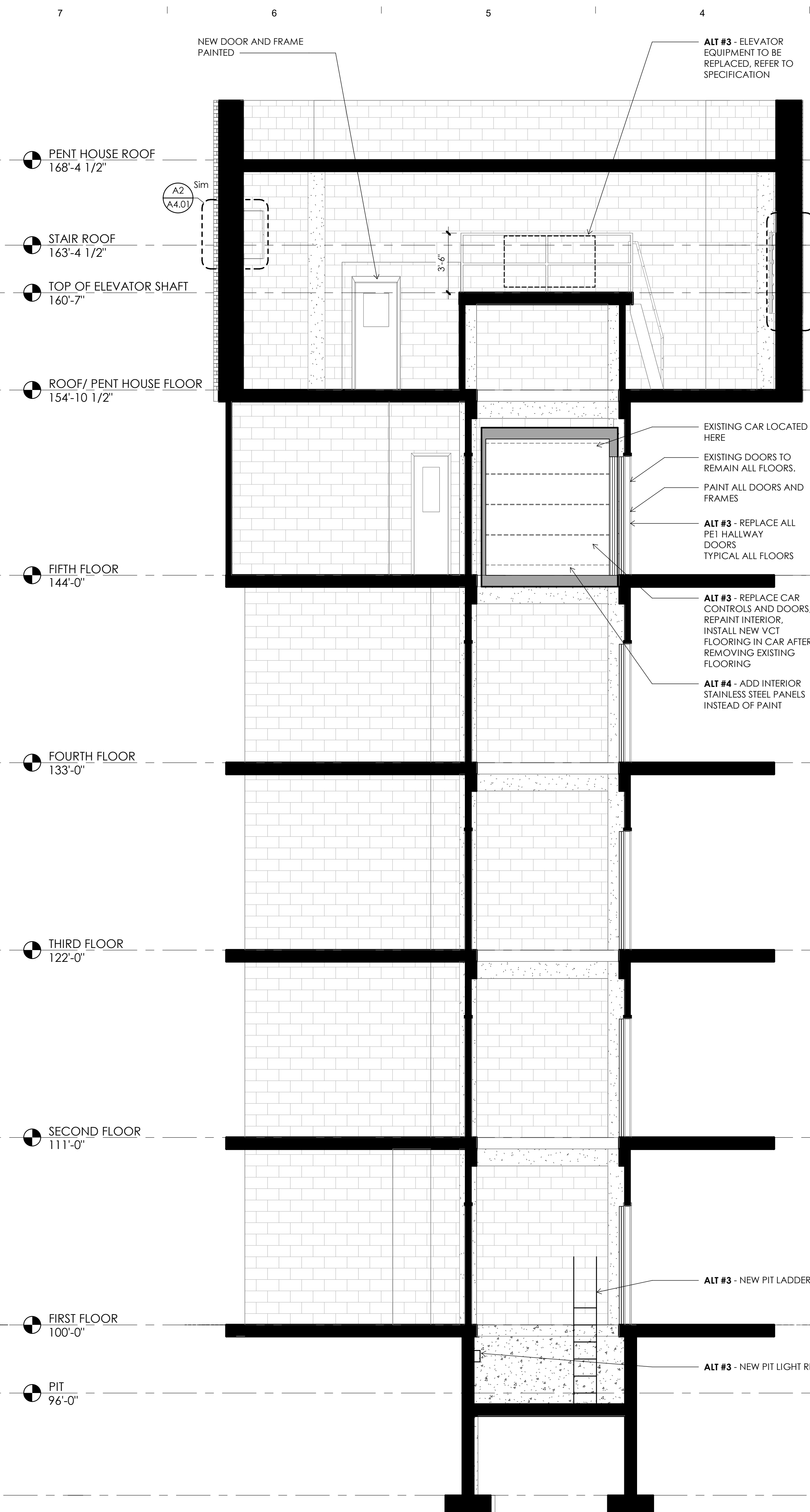
A6 PE1 ELEVATOR SECTION 1/4" = 1'-0"
