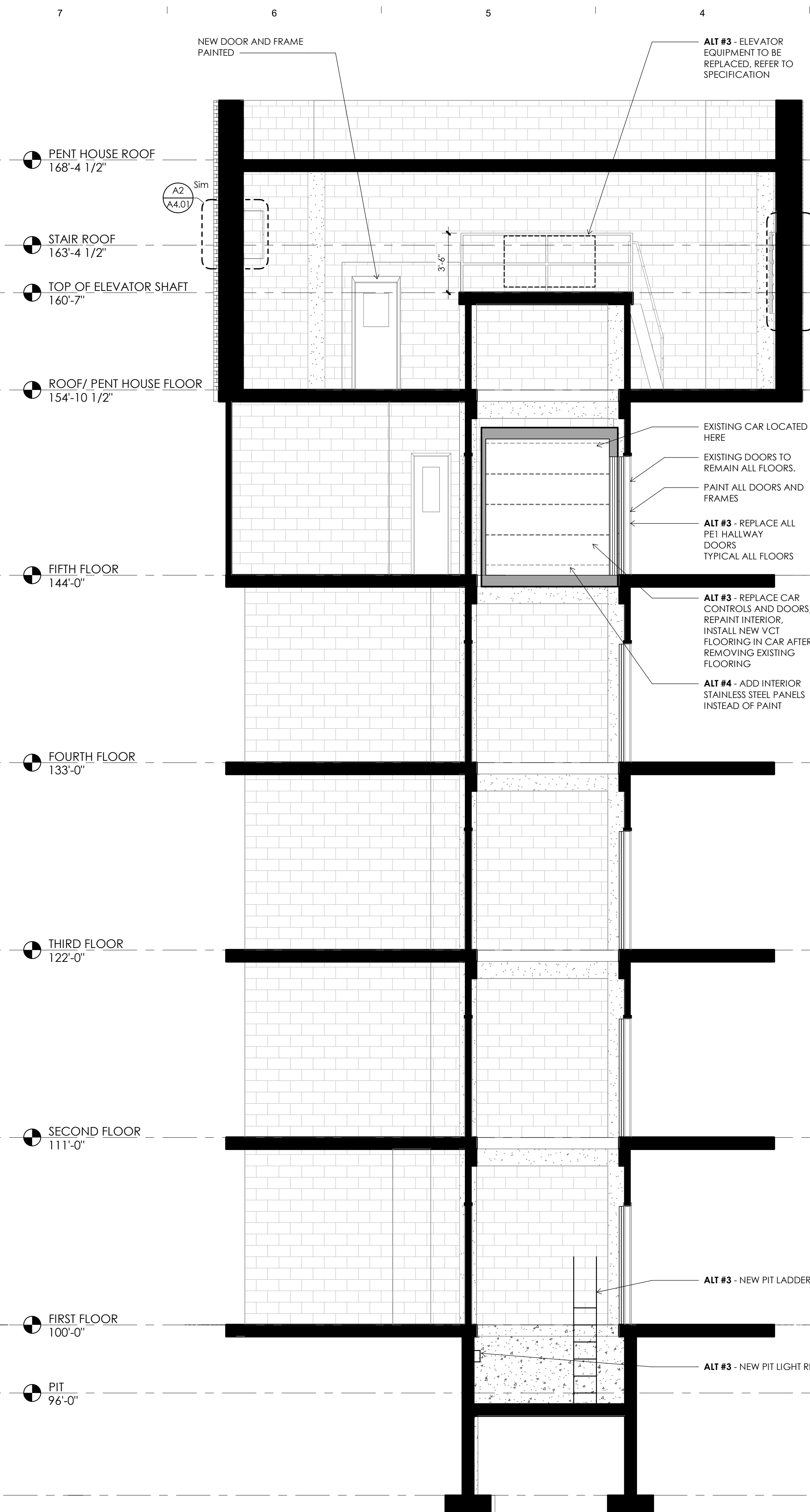
A6 PE1 ELEVATOR SECTION 1/4" = 1'-0"
