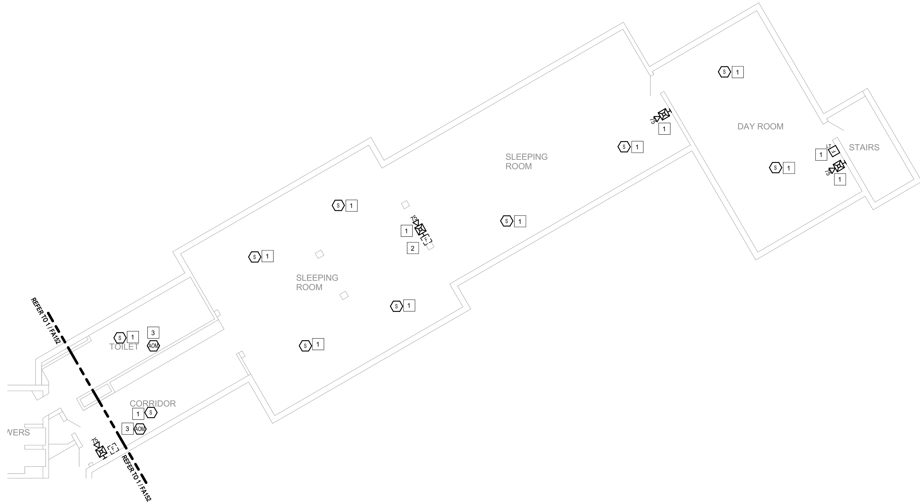
2 BUILDING 25 - LEVEL 2 - EAST WING - FIRE ALARM 1/8" = 1'-0"
