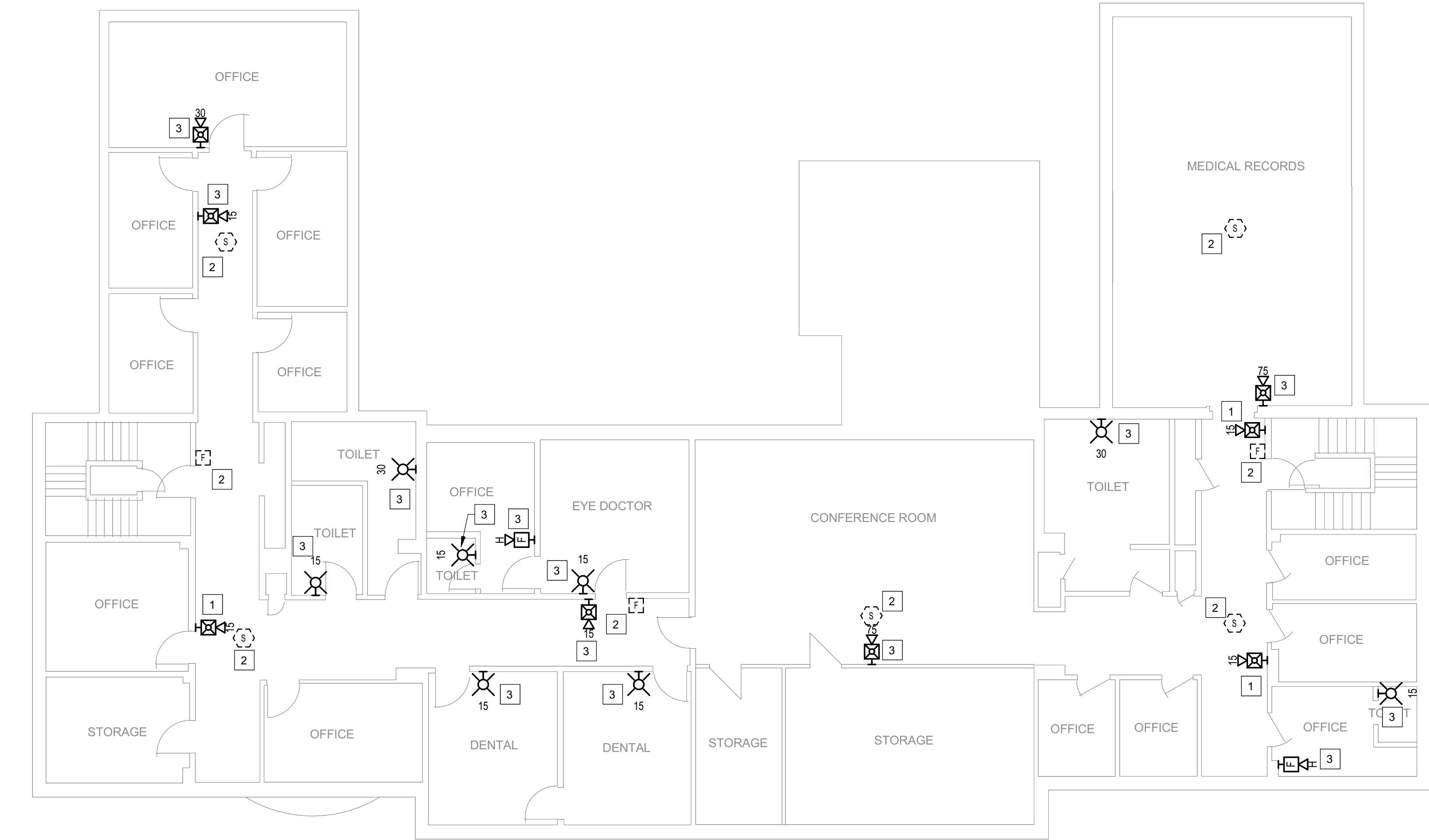
1 BUILDING 16 - LEVEL 2 - FIRE ALARM 1/8" = 1'-0"
