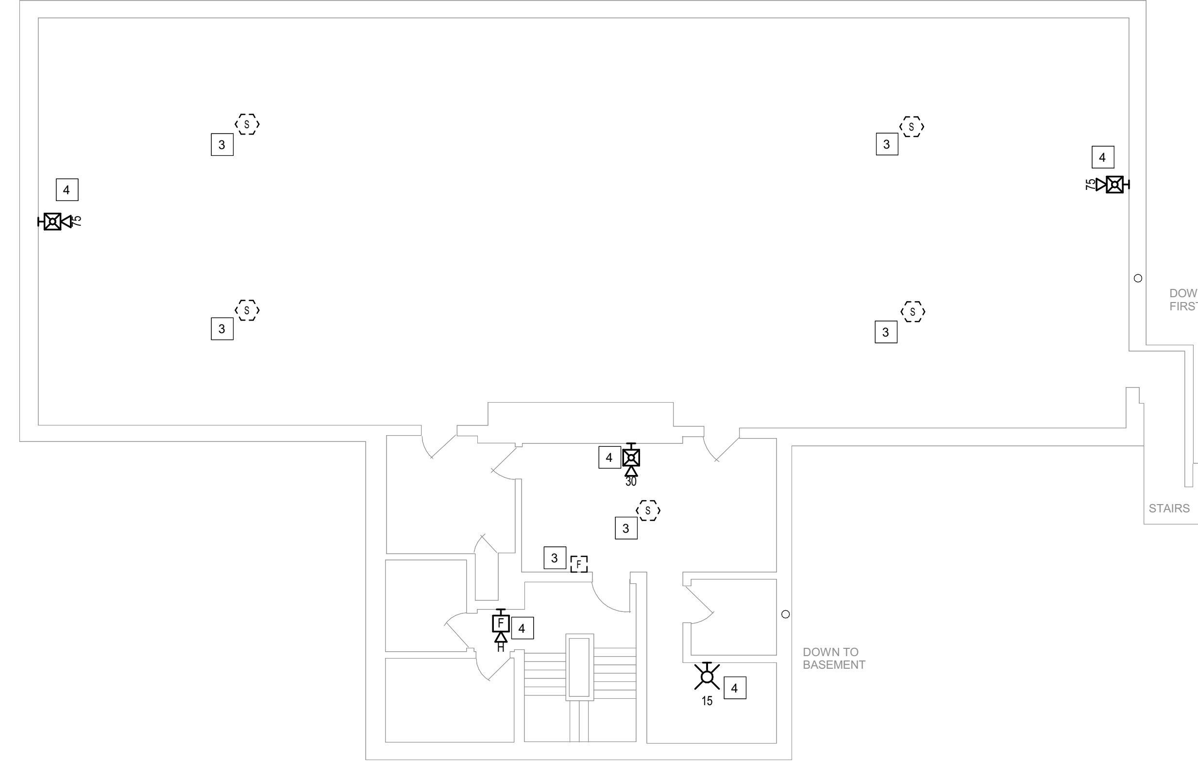
3 BUILDING 23 - LEVEL 2 - FIRE ALARM 1/8" = 1'-0"
