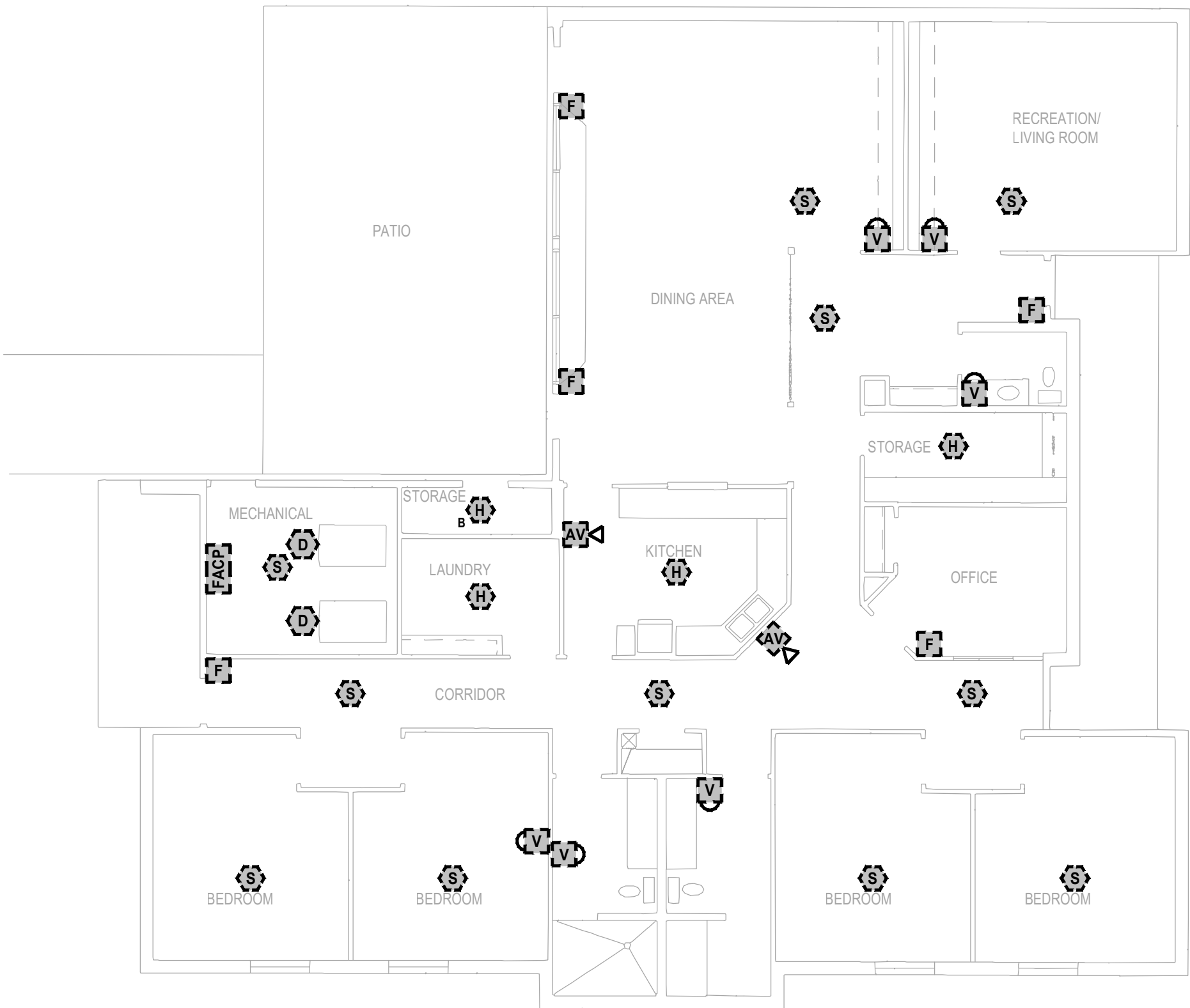
BUILDINGS 1601-1610, 1908 FIRE ALARM PLAN - DEMOLITION WORK
