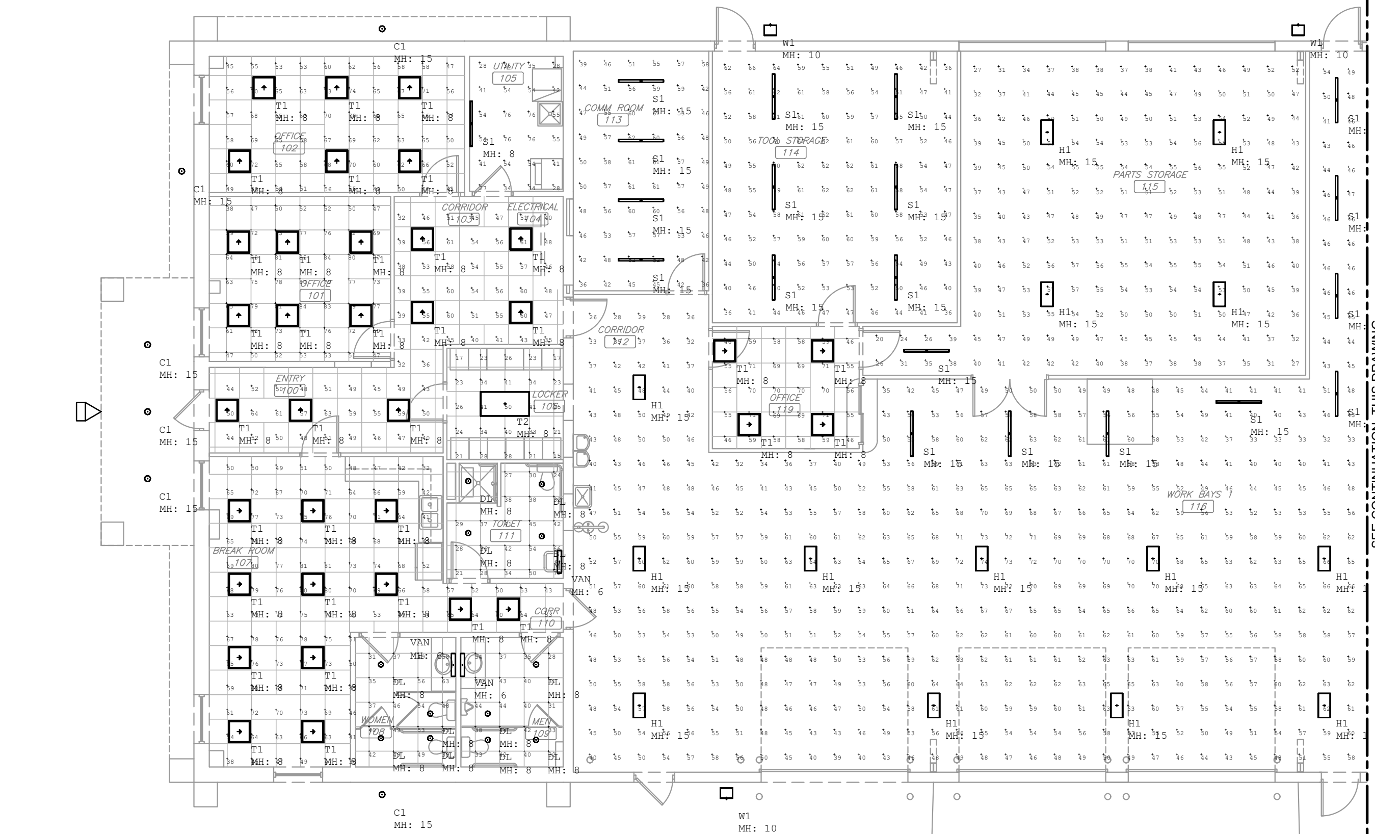
2 LUMINAIRE LAYOUT - AREA B 1/8" = 1'-0" NORTH
