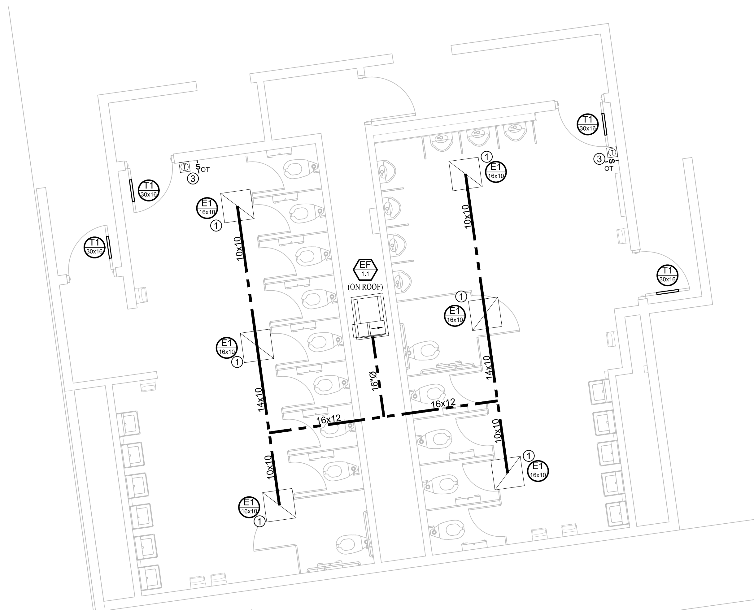
SOUTH BATHROOMS HVAC PLAN
