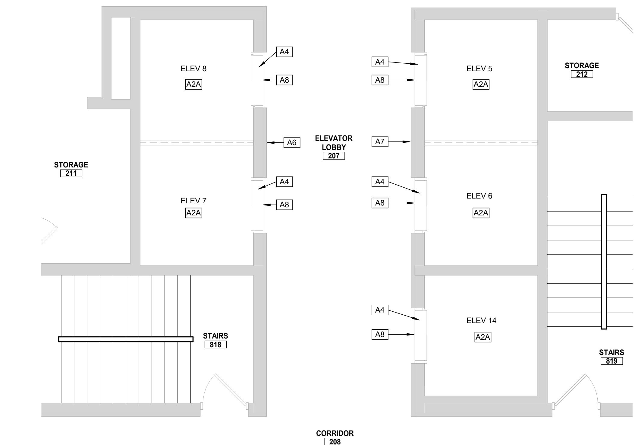
2ND FLOOR PLAN - SOUTH PASSENGER ELEVATORS 3 1/4" = 1'-0"
