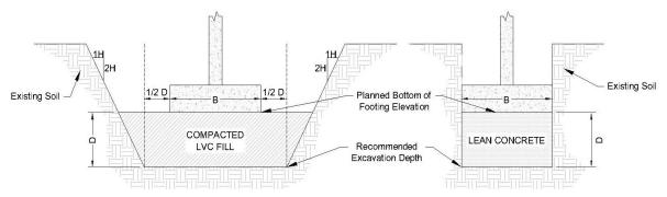
NOTE: Total excavation width to be sufficient for operation of full-size compaction equipment.
