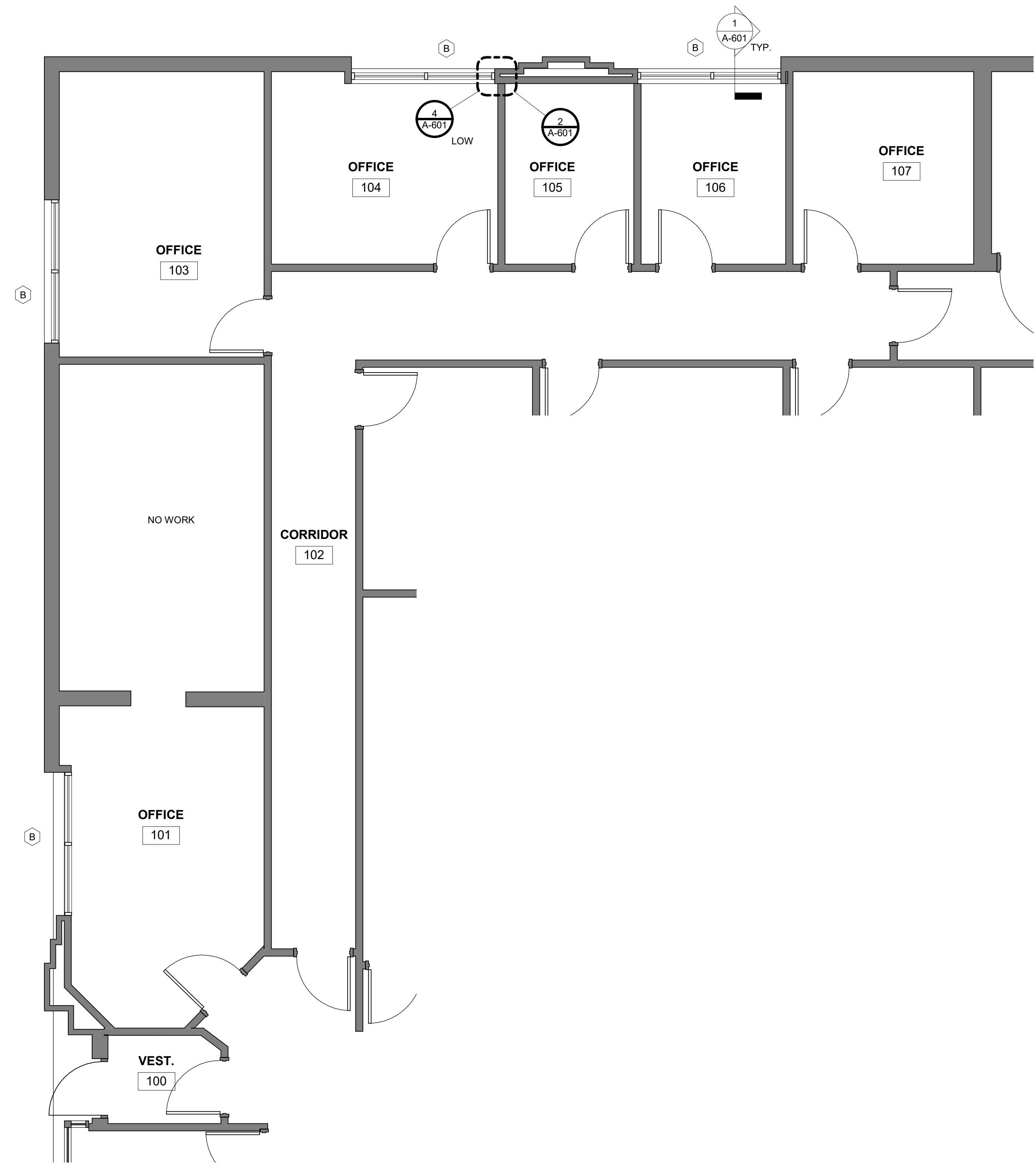
1 LEVEL 1 - ENLARGED FLOOR PLAN BASE BID SCALE: 1/4" = 1'-0"
