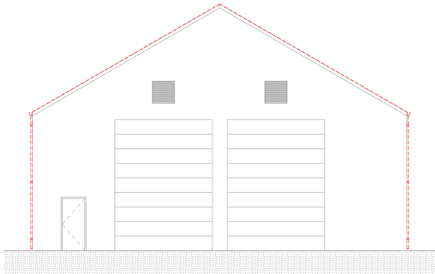
2 USB NORTH ELEVATION - DEMOLITION
