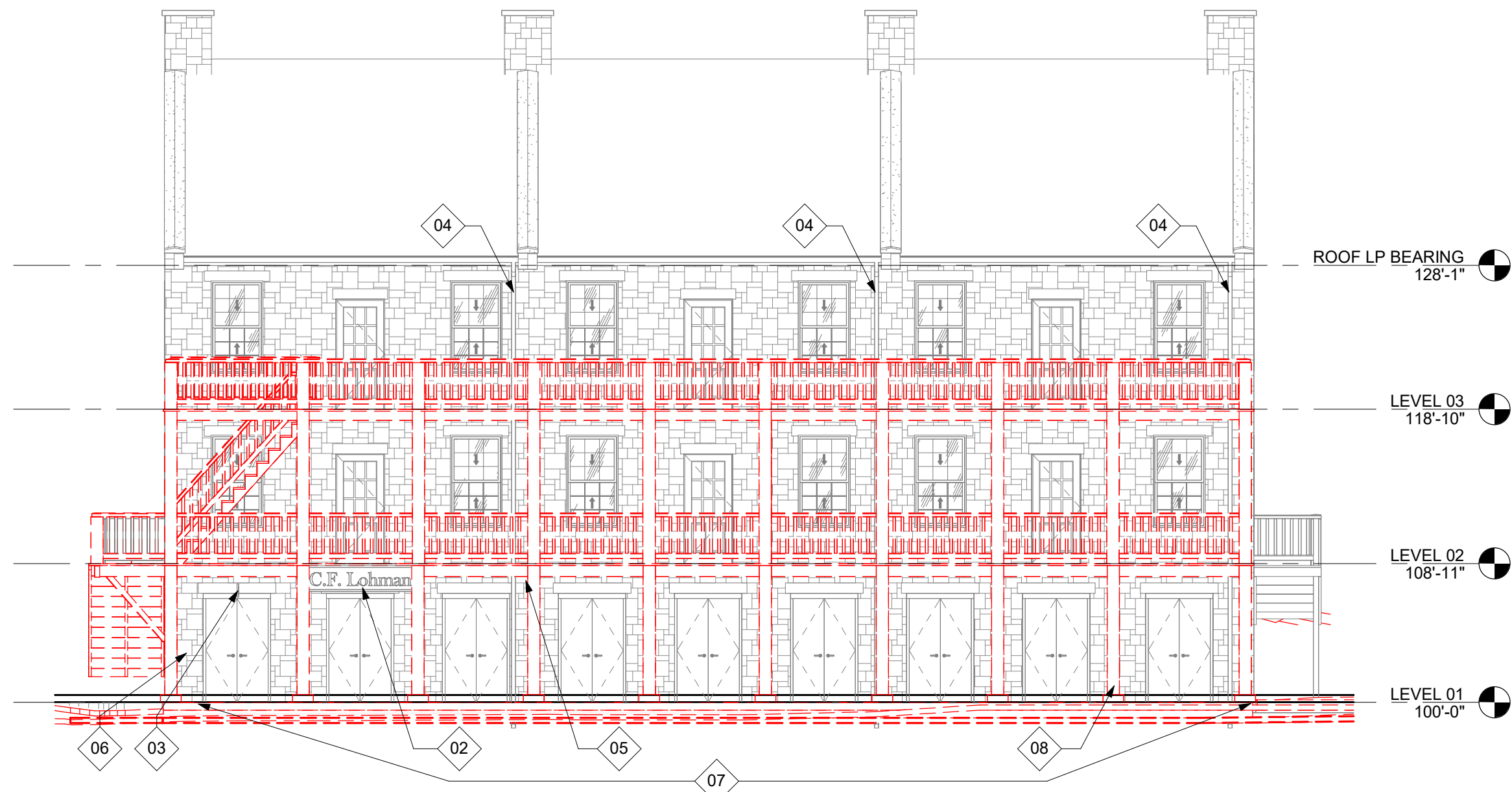
04 NORTH DEMOLITION ELEVATION
