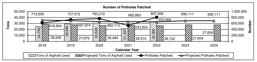
The number of potholes patched in each calendar year is estimated by the total tonnage of asphalt used during the same time period. The 2023 and 2024 projections were established by averaging the tonnage of asphalt used and number of potholes patched for the last five calendar years.
