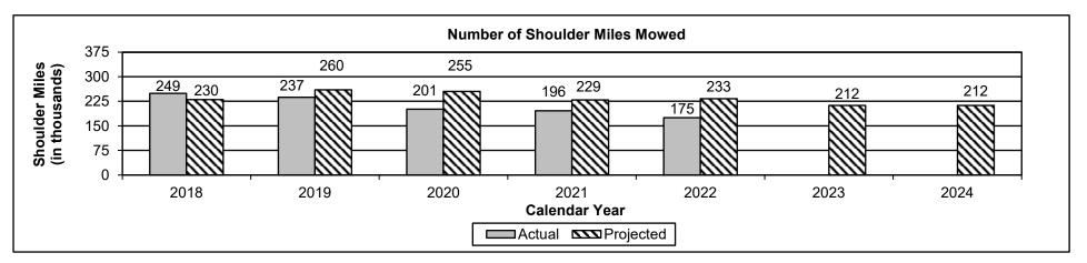
The department mows two 15 foot wide passes off the shoulder on the final mow of the season in odd numbered years, rather than one 15 foot wide pass in even numbered years. The 2023 and 2024 projections were established by averaging the number of shoulder miles mowed in the last five years.
